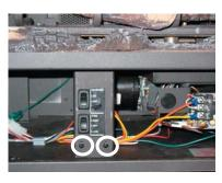
7) Remove the burner ON/OFF switch from the bracket using a pair of pliers and remove the 2 screws that secure the 2 wires on the valve.
